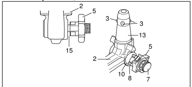
**Installation of the ball bar:**
